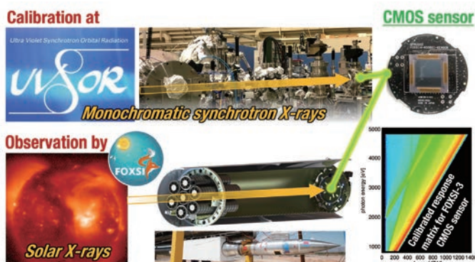
CMOS X-ray imaging sensor evaluated at BL2A
