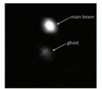
Fig. 2. Main beam and ghost image induced by  $MgF_2$  plate with the thickness of 0.5 mm at 121.6 nm with the slit width of 300 um.
