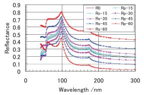
Fig. 2. Calculated spectral reflectance spectra for a diamond detector for both p- and s-components.
