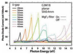
Fig. 3. Throughout spectra with some undulator gap size with and without a VUV filter,  $MgF_2$ , in the low photon-energy region.
