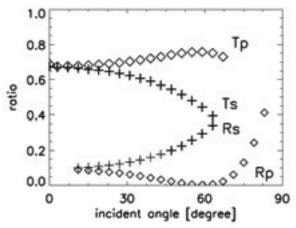
Fig. 2. Result of reflection/transmission ratio measurement.
