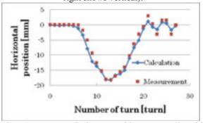
Fig. 3. Measured bump orbit compared with numerical one.
