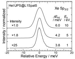
Fig. 1. Xe  $5p_{3/2}$  peak obtained by using a Gammadata VUV5000 He lamp and the A1ER-SES200 system at  $E_p = 1, 5, and 10 \text{ eV}.$
