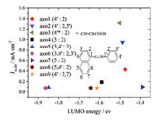
Fig. 1. Correlation between the experimental data of the short current density of DSCs and the theoretical LUMO energy levels of the solitary azo dyes. The positions of carboxylate and hydroxy groups are shown using the numbers before and after the semicolon in the parentheses, respectively.
