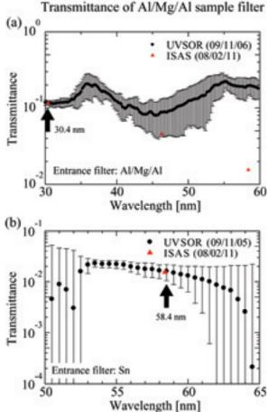
Fig. 1. The transmittances of the Al/Mg/Al sample filter measured at UVSOR and at ISAS. The Al/Mg/Al filter and the Sn filter are used as the entrance filter at UVSOR for (a) 30.4 nm and (b) 58.4 nm, respectively.
