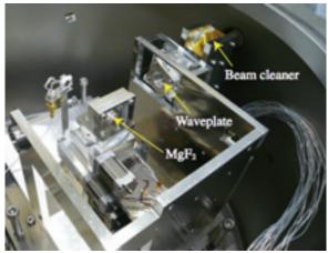
Fig. 1. Photo of our measurement system. The position of the waveplate and  $MgF_2$  plate are controlled by the stepping motors.
