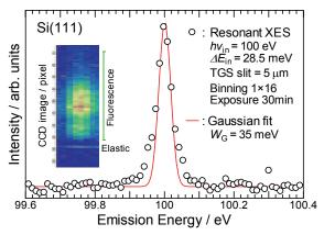
Fig. 2. Si L $\alpha$  resonant XES spectrum ( $hv_{in} = 100 \text{ eV}$ ) for the Si(111) wafer obtained by using new TG with the best fit curve using the Gaussian function with the linewidth of 35 meV.
