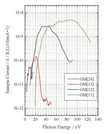
Fig. 1. Throughput spectra of plane-grating monochromator at BL8B2 (slit=100µm).
