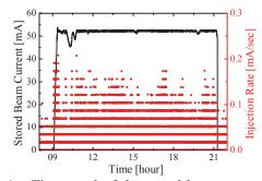
Fig. 4. Time trend of the stored beam current and injection rate during the single-bunch top-up operation in 16 Sep. 2009.
