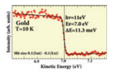
Fig. 3. HRPES spectrum at the Fermi level of gold measured after the present reconstruction.
