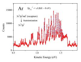
Fig. 2. Autoionization spectrum following the 2p photoionization of Ar.
