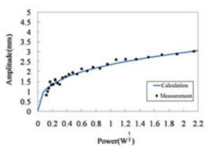
Fig. 3. Measured and calculated horizontal betatron oscillation amplitude to power.
