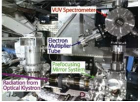
Fig. 1. Photo of VUV spectral measurement system.
