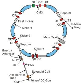
Fig. 1. Schematic drawing of UVSOR-II injector.
