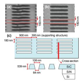
Fig. 1. SEM image for the prototype TG (a) and new TG (b) with the groove density of 6250 lines/mm (160 nm period) and 5555 lines/mm (180 nm period), respectively. (c) Basic structure of the new TG.
