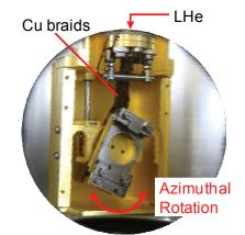
Fig. 2. Photo of the LHe 5-axes manipulator without a front radiation shield and a sample-mounting puck.
