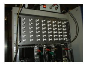
Fig. 1. Distribution board for injection signal.
