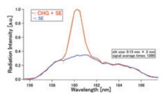
Fig. 2. Spectra of SE (blue line) and CH (red line) at the 5th harmonic.
