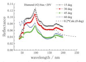
Fig. 1. Measured spectral reflectance spectra for a diamond detector (Calculated spectrum at normal incidence is also shown in dashed line).
