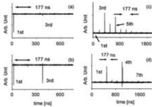
Fig. 1. CSR signals of three diode detectors at the low-alpha optics. Revolution time of the ring is 177 ns. (a), (b), and (c) are with the low-alpha (1/2) optics. Sensitivity ranges are (a)  $11.0 - 16.6 \text{ cm}^{-1}$ , (b) 7.3 -  $11.0 \text{ cm}^{-1}$ , and (c)  $3.7 - 5.7 \text{ cm}^{-1}$ . (d) is with low-alpha (1/3) optics. Sensitivity range is 7.3 -  $11.0 \text{ cm}^{-1}$ .
