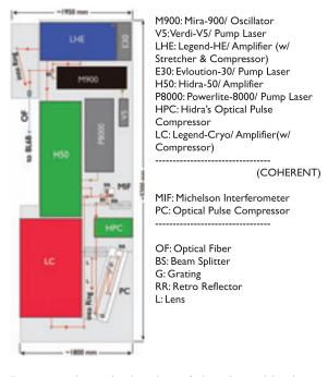
Fig. 1. A schematic drawing of the Ti:sapphire laser system.
