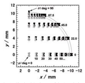
Fig. 1. Simulated 2D images of the 3D velocity distribution of  $C_{58}^+$  from  $C_{60}$  projected on the PSD. The initial kinetic energies of  $C_{58}^+$  were set to 0.1 (O) and 0.11 eV ( $\blacksquare$ ).
