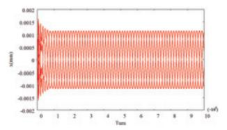
Fig. 2. Simulated horizontal beam position from center of BPM chamber every turn.
