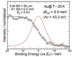
Fig. 3. Fermi edge of Au film measured at  $E_p = 5$  eV, hv = 43.2 eV, and  $T \sim 20$  K.
