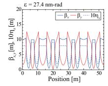
Horizontal / vertical betatron functions and dispersion function
