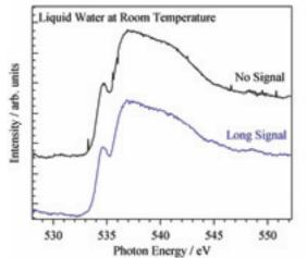
Fig. 3. Result of first application of beam injection signal (O K-edge X-ray absorption spectrum for liquid water).
