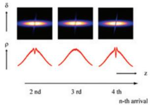
Fig. 2. An example of evolution of fragments and a dip structure in longitudinal phase space (upper) and its corresponding longitudinal density distribution (lower). The horizontal axis is an arrival order after the revolutions
