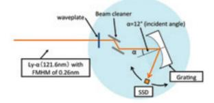
Fig 1. Setup of grating reflectivity measurement for the vertical polarization.
