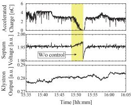
Fig. 4. Time trend of the accelerated charge in the UVSOR-II injector (top), peak voltage of the electric septum (middle) and output power for the accelerator tube (bottom) with and without the stabilization.
