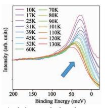
Fig. 2. Angle-integrated photoelectron spectra of YbCu<sub>2</sub>/Cu(111) taken at hv = 37 eV (T = 10~130 K). The allow indicates the Kondo resonance peak.
