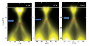
Fig. 1. Band dispersion image of the MnBi<sub>2</sub>Te<sub>4</sub>/ MnBi<sub>2</sub>Te<sub>4</sub>/Bi<sub>2</sub>Te<sub>3</sub>/MnBi<sub>2</sub>Se<sub>4</sub> hetero structure measured at 6.6 K, 160 K, and 250 K, respectively.
