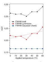
Fig. 2. Influence of temperature on the width of the main line (full width at half maximum: FWHM). The Gaussian and Lorentzian contributions are extracted.
