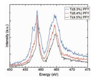
Fig. 1. Ti  $L_{2,3}$ -edge X-ray absorption spectra of  $Al_{1-x}Ti_xN$  films (x= 0.083, 0.064, and 0.045) These spectra were measured in partial fluorescence yield (PFY) mode.
