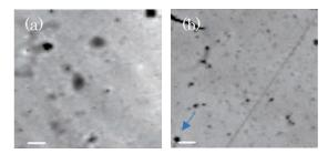
Fig. 1. X-ray absorption image of (a) unvulcanized and (b) vulcanized rubbers taken at 400 eV. Scale bars are 5  $\mu$ m.
