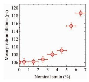
Fig. 2. Change in mean positron lifetime during tensile deformation.
