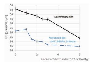
Fig. 3. GD of electron beam tracks. The solid and dashed lines show the data of unrefreshed films and refreshed films, respectively.
