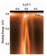
Fig. 1. ARPES band dispersion of YbCu<sub>2</sub>/Cu(111) surface along  $\overline{\Gamma}$ - $\overline{K}$  taken at hv = 37 eV (T = 7 K). The photoelectron intensities were normalized by the Fermi-Dirac distribution function convoluted with the instrumental resolution.
