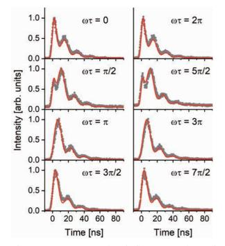
Fig. 1. Zeeman quantum beat in fluorescence decay of helium atoms [4]. The quantum phase  $\omega \tau$  is set to increase from 0 to  $7\pi/2$  with a step size of approximately  $\pi/2$  where  $\omega$  is the resonance frequency from the ground state to the 1s6p state. The experimental data points are shown by gray circles and the red curves represent the calculation results
