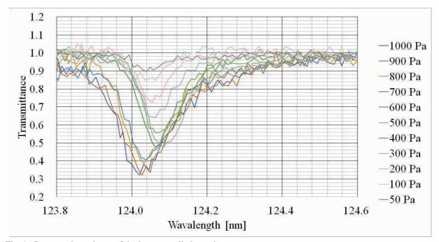
Fig. 1. Pressure dependence of the krypton cell absorption.
