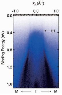
Fig. 2. ARPES intensity plot of  $CeTe_{1.83}Sb_{0.17}$  along  $\Gamma$ -M taken with 103 eV at 15 K.
