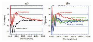
Fig. 2. CD spectra of alanine sample after irradiation of (a) right (red) and left (black)-CPL, and (b) right CPL with magnetic field application (blue:+0.7T, green:-0.7T).
