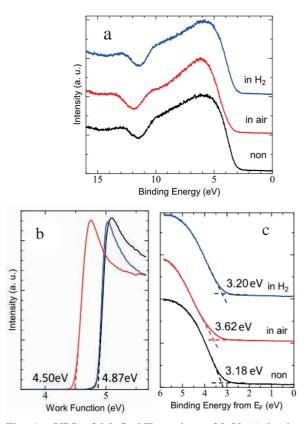
Fig. 1. UPS of  $MoO_3$  NPs at hv = 28eV (a) in the valence band region (b) in the secondary cut-off and (c) in the valence top region.
