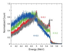
Fig. 3. Measured LCS beam spectra with the undulator K-value of 0, 0.1, 0.2, and 0.3.
