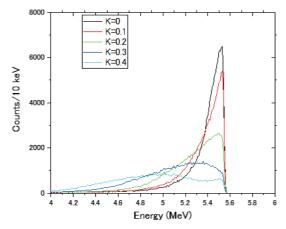
Fig. 2. LCS gamma-ray energy distribution in the vertical axis with the undulator K-value of K=0.2.
