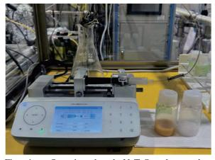
Fig. 1. Strontium-doped  $NaTaO_3$  photocatalyst particles suspended in water. White suspension in the syringe was sent to the liquid film cell for transmission XAFS measurements.
