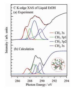
Fig. 1. C K-edge XAS spectra of liquid EtOH from (a) experiments and (b) calculations. The inset shows one of the liquid structures used for the inner-shell calculations, where EtOH molecules were extracted from the liquid structure within the  $CH_2$ - $CH_2$  distance of 6 Å from the central EtOH molecule.
