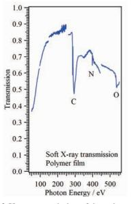
Fig. 1. Soft X-ray transmission of the polymer film.
