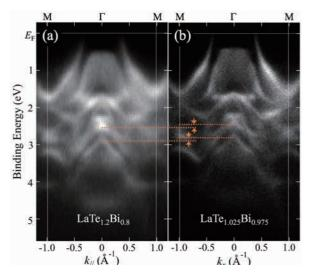
Fig. 1. Comparison of ARPES intensity maps along the  $\Gamma$ -M direction of LnTe<sub>1+x</sub>Bi<sub>1-x</sub> between (a) x = 0.2 and (b) x = 0.025, measured with 94 eV photons and at 20 K.
