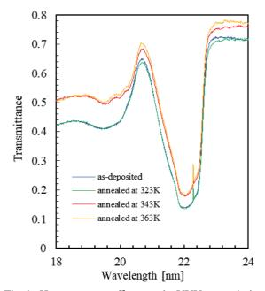
Fig. 1. Heat treatment effects on the VUV transmission spectrum of amorphous selenium film.
