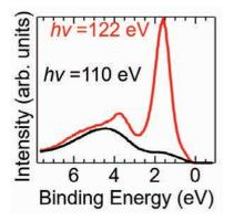
Fig. 1. Resonant angle-integrated photoelectron spectra of  $CeTe_{1.83}Sb_{0.17}$  at 15 K. The excitation energies of 110 and 122 eV correspond to the off- and on-resonance conditions at the Ce 4*d*-4*f* absorption edge.
