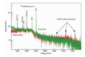
Fig. 2. Typical  $\gamma$ -ray spectra observed for <sup>208</sup>Pb before (red) and after (green) heavy shield. NRF levels are labeled with resonance energies. Also, single and double escape peaks are labeled. The high energy background was effectively suppressed.
