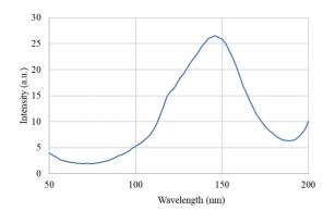
Fig. 3. Excitation spectrum of the plastic scintillators having DPO-POPOP concentration of 2 wt%.
