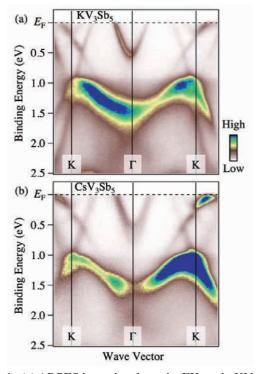
Fig. 1. (a) ARPES intensity along the  $\Gamma$ K cut in KV<sub>3</sub>Sb<sub>5</sub> plotted as a function of binding energy and wave vector. (b) Same as (a) but for CsV<sub>3</sub>Sb<sub>5</sub>.
