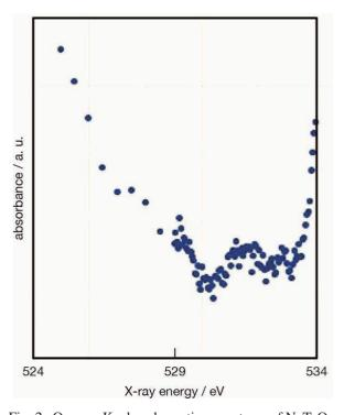
Fig. 2. Oxygen K edge absorption spectrum of  $NaTaO_3$  photocatalyst particles doped with Sr cations observed in water without UV light irradiation. The absorbance spectrum is shown in an arbitrary unit as a function of X-ray energy.
