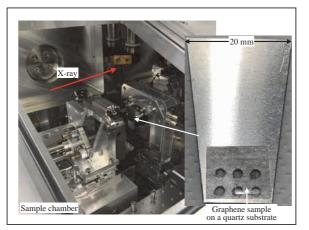
Fig. 1. Sample chamber and a close-up view of the graphene sample on the quartz substrate with a taper structure.
