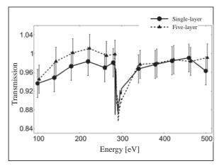
Fig. 2. Resultant transmission from 100 to 500 eV for single- (filled circle) and five-layer (triangle) graphene samples (Kashiwakura, Mitsuishi *et al.*, in prep.). Systematic errors are  $\pm/-3\%$ .
