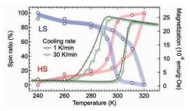
Fig. 2. The spin state wight of  $Fe^{2+}$  ions as the function of the temperature.
