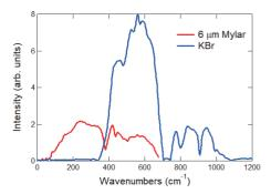
Fig. 2. Obtained intensity spectra with the combination of a light source (UVSOR), detector (Si bolometer), and interferometer (Bruker Vertex70v) with different beamsplitters (6  $\mu$ m Mylar and KBr). (Only low energy side is shown).
