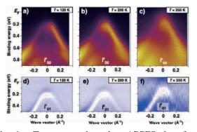
Fig. 1. Temperature-dependent ARPES data from  $Ta_2Ni(Se_{1-x}S_x)_5$  at  $x \sim 0.6$  measured at (a)  $T \sim 120$  K, (b) 200 K and (c) 350 K. The second derivative plots from  $\Gamma_{01}$  are shown on the bottom panel (d-f).
