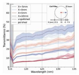
Fig. 1. Transmission spectra of MgF2 windows on a hydrogen absorption cell.
