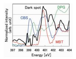
Fig. 2. N *K*-edge NEXAFS spectra of CBS (blue), DPG (green), MBT (red) and a dark spot (shown in Fig. 1 by an arrow). The spectra are normalized by max and minimum.
