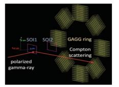
Fig. 1. Two SOI sensors and eight GAGG arrays are used to detect polarized gamma-rays.
