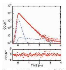
Fig. 1. (Upper) GiPALS spectrum of a  $\beta$ -SiALON:Eu phosphor. (Lower) Residual between the results of experiment and curve fit analysis.
