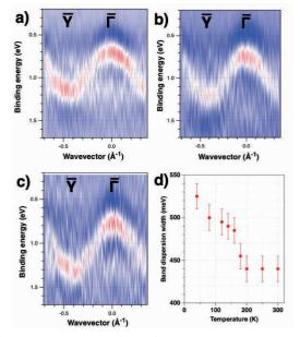
Fig. 1. Temperature-dependent ARPES data (second derivative plots) obtained along the  $\Gamma$ -Y direction at (a) T = 300 K, (b) 180 K and (c) 80 K. (d) shows the band dispersion widths as a function of temperature extracted from our measurements.
