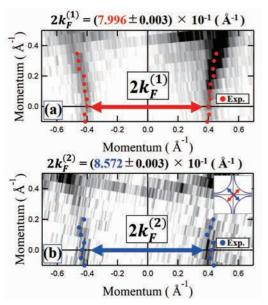
Fig. 1. (a), (b) Fermi surface mapping obtained by rotating around the two nodal directions taken at hv = 60 eV and T = 20 K with the *s*-polarization geometry. Red and blue markers indicate the Fermi surface points determined from the peaks of the momentum distribution curves. We determine  $2k_{\rm F}$  values ( $2k_{\rm F}^{(1)}$  and  $2k_{\rm F}^{(2)}$ ) for the two nodal directions as shown in the inset of panel (b).
