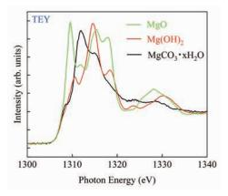
Fig. 1. Mg *K*-edge NEXAFS spectra of MgO, Mg(OH)<sub>2</sub> and MgCO<sub>3</sub>  $\cdot$  xH<sub>2</sub>O powder obtained from TEY mode.
