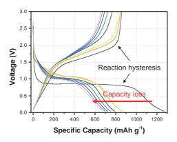
Fig. 1. Charge/discharge profiles of the synthesized  $\alpha$  -Fe<sub>2</sub>O<sub>3</sub> at 0.1 C current rate. (Unpublished)
