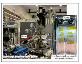
Fig. 1. Sample chamber and a close-up view of the graphene sample on the quartz substrate.
