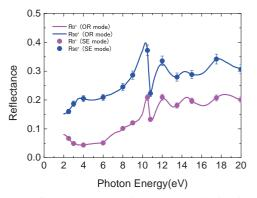
Fig. 1. Reflectance spectra in *p*- and *s*-polarization configurations of fused quartz glass
