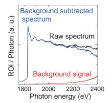
Fig. 2. Si K-edge XAFS Spectra for the deposited Ta@  $Si_{16}$  SA samples. The spectrum in blue was obtained by subtracting background signal in red from raw spectrum in black. The spectrum in 1800-2000 eV was used for the structural analyses.
