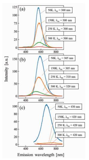
Fig. 1. Photoluminescence spectrum at each temperature for (a)  $Li_2ZrCl_{6}$  (b) $Li_2ZrBr_{6}$ , (c) $Li_2ZrI_{6}$
