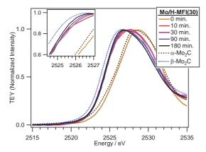
Fig. 2. Mo  $L_{III}$ -edge XANES spectra of Mo/H-MFI (Si/Al<sub>2</sub>=30) catalyst after the reaction for each time (0 – 180 minutes).
