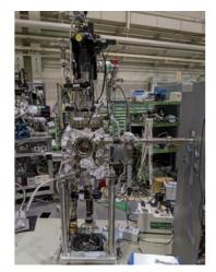
Fig. 2. The vacuum chamber for the maeasurements in UVSOR BL4B.
