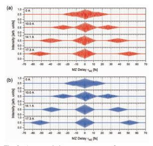
Fig. 2. Autocorrelation measurements of spontaneous radiation from the tandem undulator at various values of the phase shifter current. The wavelength of the fundamental undulator radiation was set to 357 nm. (a) Measurement. (b) Calculation.
