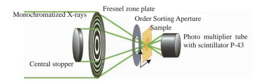
Fig. 2. Schematic image of STXM
