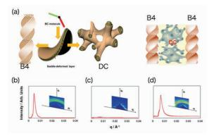
Fig. 1. (a) Schematics of the nanoscopic structures of the B4 and DC phases, and the nano-separated dual chiral phase. (b, c, d) RSoXS patterns obtained for (b) B4, (c), DC, and (d) dual chiral phases. [2]
