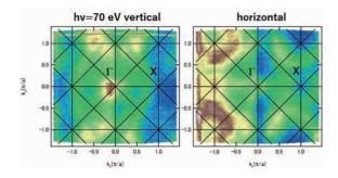
Fig. 1. ARPES images of  $Mn_3Ga$  taken at hv=70 eV using (a) *s*-polarized beam and (b) *p*-polarized beam.
