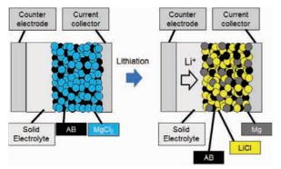
Fig. 1. Schematic view of "in-situ forming of solid electrolyte" in  $MgCl_2$  electrode using  $Li/LiBH_4/MgCl_2$  cell.
