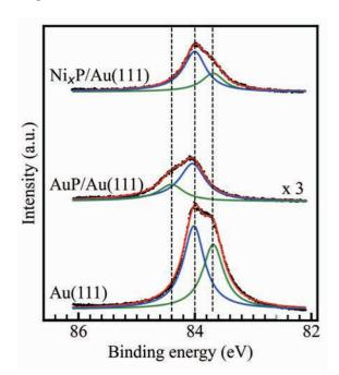
Fig. 1. Au  $4_{7/2}$  photoelectron spectra of clean Au(111), AuP/Au(111) and NiP/Au(111) samples.
