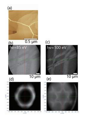
Fig. 1. (a) AFM image and (b)-(c) PEEM images of graphene/Ir(111). Iso-energy cross sections of 2D band dispersion of graphene/Ir(111), with photon energy of (d) 85 eV and (e) 100 eV.
