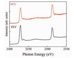
Fig. 2. Zr *L*-edge NEXAFS spectra of  $ZrO_2$  powder obtained from TEY and PFY.
