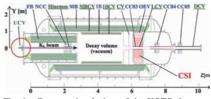
Fig. 1. Cross-sectional view of the KOTO detector. The beam enters from the left. Detector components with their abbreviated names written in blue (in green and underlined) are photon (charged-particle) veto counters. The UCV detector is installed at the upstream (left) end of the KOTO detector.
