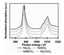
Fig. 1. Nd  $M_{4,5}$ -edge XANES spectra of Nd complex oxides
