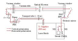
Fig. 1. Schematics of laser transport line and light measurement setup.
