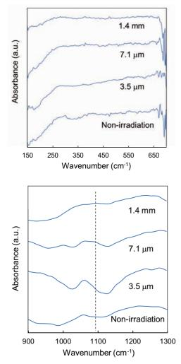
Fig. 1. Infrared absorption spectra of lignin in the far-(upper) and mid-(bottom) infrared regions. "1.4 mm" means the wavelength of submillimeter wave from gyrotron. Both of "7.1 µm" and "3.5 µm" are wavelengths of IR-FELs.
