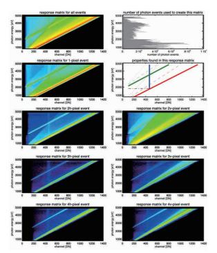
Fig. 1. Measured response matrix of the FOXSI-3 CMOS detector from 840 eV to 4500 eV. In the color maps, the horizontal axis shows the values of output signals from the detector, when the detector detects the monochromatic X-ray photons with the energy shown in the vertical axis. The colors indicate, in log scale, how frequently each signal value is output. The top-right panel shows the number of monochromatic X-ray photons used to create this matrix.
