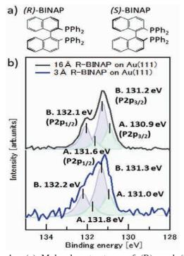
Fig. 1. (a) Molecular structures of (R)- and (S)-BINAPs. (b) P2p core level peaks of (R)-BINAP on Au(111) measured by XPS at the nominal coverages of 0.4 ML (bottom) and 2 ML (top). The spectra at each coverage are fitted with the two spin-orbit doublets [labelled A (green) and B (blue)] with Doniach-Sanjic lineshape.
