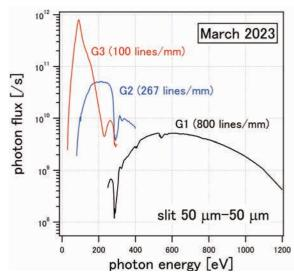
Fig. 1. Photon flux curves for G1, G2 and G3. Entrance and exit slits are set to 50 µm.
