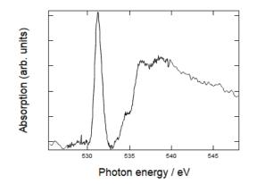
Fig. 1. O-K XAS spectrum for  $Mo(CO)_6$  (40 mg) in 10 ml CH<sub>3</sub>CN at room temperature.
