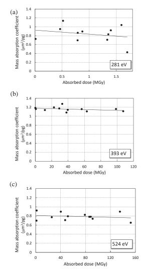
Fig. 1. Effects of soft X-rays on mass absorption coefficients in DNA at (a) C K, (b) N K, (c) O K- edges. The solid lines show linear regression.
