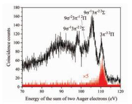
Fig. 2.  $OCS^{3+}$  spectra formed by the S2p double Auger decay of OCS: total spectrum (black solid curve) and the one filtered with further coincidence with parent  $OCS^{3+}$  ions (red shaded spectrum).
