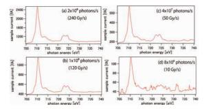
Fig. 2. TEY spectra of FePO<sub>4</sub> powders for various photon fluxes.
