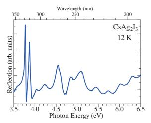
Fig. 1. Reflection spectrum of the  $CsAg_2I_3$  crystal at 12K.
