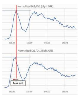
Fig. 2. Oxygen K edge absorption spectrum of a Srdoped NaTaO<sub>3</sub> photocatalyst disk in the absence (upper panel) and presence (lower panel) of UV-light irradiation.
