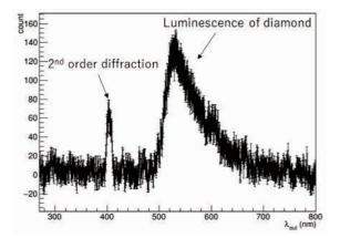
Fig. 2. Photoluminescence spectrum of a commercially available HPHT diamond measured by using the system shown as Fig.1. Ultra violet light with wavelength of 200 nm was used for photoluminescence excitation.
