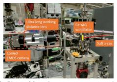
Fig. 2. Photo of focus image measurement equipment at an endstation of BL4B.
