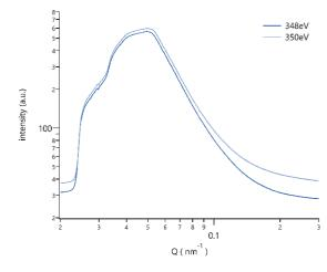
Fig. 1. Q-spectra for casein at the calcium L absorption edge.
