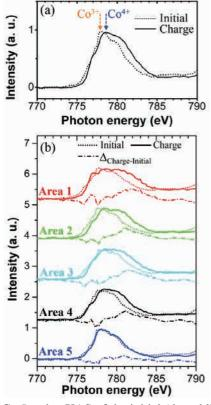
Fig. 1. Co  $L_3$ -edge XAS of the initial (dotted line) and charged (solid line) conditions of LCO. Panel (a) shows average spectra of selected particles including area 1-5 (circle areas: 300 nm diameter). Panel (b) shows extracted spectra from area 1-5, which exhibit different charging states (oxidation states) from each other.
