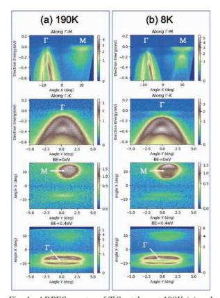
Fig. 1. ARPES spectra of  $TiSe_2$  taken at 190K (a) and 8K (b). Upper two panels for (a) and (b) show the intensity maps along the energy-angle axes. Lower two show the iso-energy intensity maps along the x- and y-angles at the binding energies of 0eV and 0.4eV.
