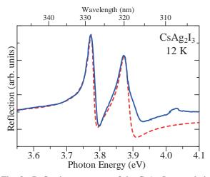
Fig. 2. Reflection spectrum of the  $CsAg_2I_3$  crystals in the band-edge exciton region at 12 K. Broken curve is the fitting result calculated with the two-oscillator model.
