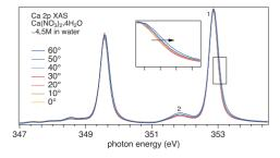
Fig. 1. X-ray absorption spectra of a  $4.5 \text{ MCa}(\text{NO}_3)_2 \cdot 4(\text{H}_2\text{O})$  aqueous solution, recorded in the vicinity of the Ca 2*p* ionization threshold, for temperatures in the 0-60°C range.
