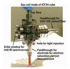
Fig. 1. A gas cell for the photoionization experiments.
