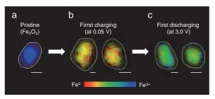
Fig. 2. Chemical composition maps at **a**. pristine, **b**. first charged state (0.05 V vs. Li/Li<sup>+</sup>), and **c**. first discharged state (3.0 V vs. Li/Li<sup>+</sup>). Scale bars below each image are 1 um.
