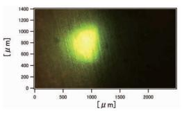
Fig. 3. Focus image at the Ce:YAG scintillator. The photon energy is 400 eV.
