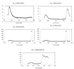
Fig. 1. PL spectra and PLE spectra of fluorite.
