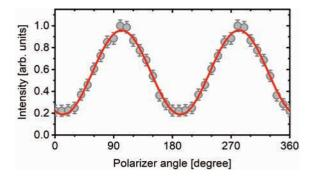
Fig. 2. Fluorescence intensity measured as a function of the polarizer angle. The experimental data points are fitted by a theoretical curve.
