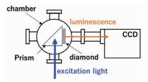
Fig. 1. A design of the experimental setup for photoluminescence measurement of diamond.
