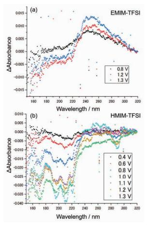
Fig. 1. Difference spectra of C9-DNBDT-NW films with (a) EMIM-TFSI and (b) HMIM-TFSI as a function of the applied voltage.
