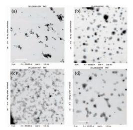
Fig. 1. The morphology of BBA particles from burning different biomasses: (a) Softwood burned under flaming condition; (b-d) softwood, peat and leaves burned under smoldering conditions, respectively. The used photon energy was 300 eV.
