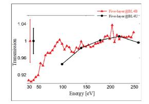
Fig. 2. Resultant transmission from 30 to 250 and from 100 to 250 eV for five-layer graphene samples measured at BL4B (filled triangle) and BL4U (filled circle) (Kashiwakura, Mitsuishi *et al.*, in prep.). Systematic errors are 5% / 3% at BL4B / BL4U.
