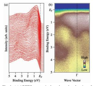
Fig. 1. (a) ARPES spectra in the valence band region of bulk  $Cr_2Se_3$  measured at T = 30 K with 21-eV photons, and (b) corresponding intensity plot as a function of binding energy and wave vector.
