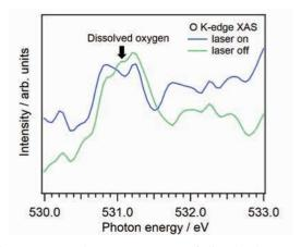
Fig. 1. O K-edge XAS spectra of dissolved oxygen, whose peak positions are around 531 eV, on lipid bilayers. The green and blue lines are the ground state (laser off) and the state under laser irradiation (laser on), respectively.
