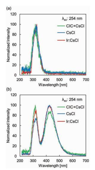
Fig. 1. Photoluminescence spectra of  $Cs_2IrCl_6$ -CsCl composite (represented as CIC+CsCl), CsCl and Ir:CsCl at (a) 300K and (b) 10K.
