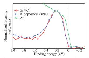
Fig. 2. Angle-integrated spectra near  $E_{\rm F}$  of ZrNCl before and after K deposition, compared with Au.
