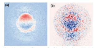
Fig. 2. Photoelectron circular dichroism (PECD) images of s-methyl oxirane measured with (a) analog integration mode and (b) counting integration mode. The propagation direction of the photoionization radiation is vertical in the figures.
