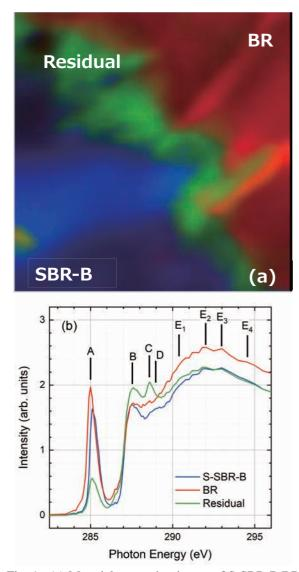
Fig. 1. (a) Material separation image of S-SBR-B/BR interface sample, (b) NEXAFS spectra of each material obtained in (a).
