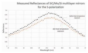
Fig. 1. Reflectances of SiC/Mo/Si mirrors before (black dots) and after (orange dots) heat-temperature exposure.
