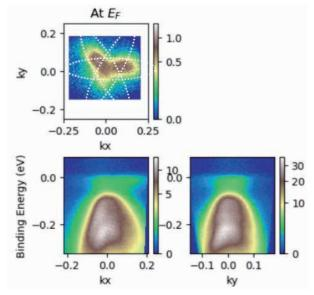
Fig. 1. ARPES spectra of  $TiSe_2$  at 10K. The photon energy taken was 7eV of vertical polarization.
