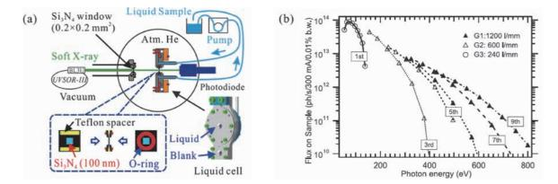
Fig. 1. (a) Schematics of a liquid cell for XAS in transmission mode settled in BL3U. The blowup shows a thin liquid layer assembled by two  $Si_3N_4$  membranes with the thickness of 100 nm. (b) Flux at the sample position with the resolving power of  $\lambda/\Delta\lambda=10^4$ .
