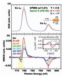
Fig. 1. (a) XAS spectrum at the Co  $L_{2,3}$  edge obtained by using the photon helicity parallel ( $\mu^+$ , red) and antiparallel ( $\mu^-$ , blue) to the external magnetic field H, respectively. (b) External magnetic field dependence of XMCD spectra ( $\mu^+-\mu^-$ ) for CPMN (x=1.01) at *T* = 4 K. Inset shows the field dependence of topological Hall effect [6].
