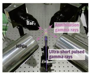
Fig. 1. Detector arrangement of GiAMOC.
