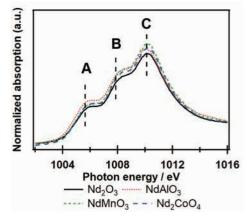
Fig. 2. Nd  $M_4$ -edge XANES spectra of Nd complex oxides
