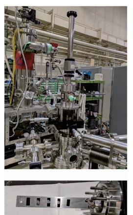
Fig. 1. The experimental setup at BL4B and the sample holder for C K-edge XAFS mesurement.
