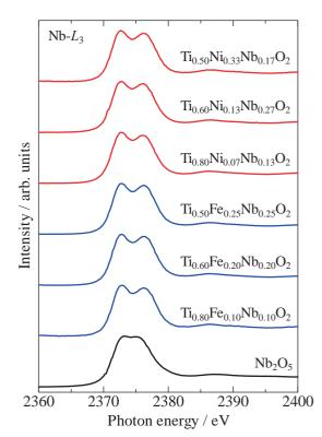
Fig. 1. Nb- $L_3$  XANES spectra of (Fe, Nb) and (Ni, Nb) co-doped TiO<sub>2</sub>.
