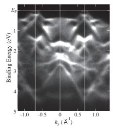
Fig. 1. ARPES intensity map of  $LaTe_{1+x}Bi_{1-x}$  measured with 94 eV photons and at 20 K.
