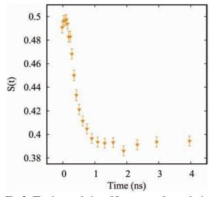
Fig. 2. The time evolution of S-parameter for synthetic silica glass.
