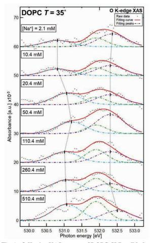
Fig. 1. O K-edge XAS spectra of DOPC-SLB at  $[Na^+] = 2.1 - 510.4$  mM obtained at the X-ray incident angle of 35°. Black dotted curves represent raw data. Dashed curves and red solid curves show deconvoluted components and their summation, respectively.
