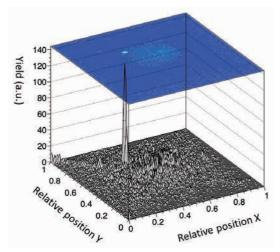
Fig. 1. Position reconstruction on the resistive anode.
