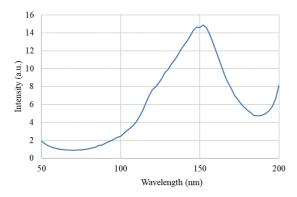
Fig. 2. Excitation spectrum of the plastic scintillators having DPO-POPOP concentration of 0.5 wt%.
