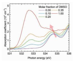
Fig. 1. The soft X-ray absorption spectra of liquid water and DMSO aqueous solutions measured for a series of molar fractions of DMSO. The spectrum of the liquid DMSO is also shown for comparison.
