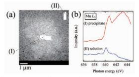
Fig. 2. (a) Mn  $L_3$ -edge STXM image and (b) spectra of selected area in the charged Ti-Mn electrolyte of the positive electrode [3].
