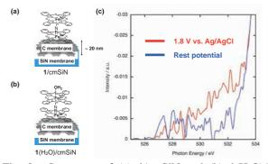
Fig. 2. Structures of (a) 1/cmSiN and (b)  $1(\text{H}_2\text{O})/\text{cmSiN}$ . (c) Comparison of O K-edge XAS spectra of  $1(\text{H}_2\text{O})/\text{cmSiN}$  at rest potential (blue) and  $1(\text{H}_2\text{O})/\text{cmSiN}$  at the applied potential of 1.8 V vs. Ag/AgCl.
