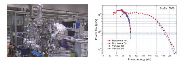
Fig. 1. Picture and photon flux of BL5U.
