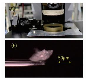
Fig. 2. (a) Photograph of the goniostage mounted on the microscope. (b) Micrograph of a sample glued to the tip of the capillary.
