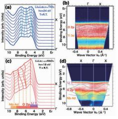
Fig. 1. ARPES spectra (a,c) and band structures (b,d) along the  $\Gamma X$  line of  $Li_{3x}La_{2/3-x}TiO_3$  (a,b) and  $Li_xLa_{(1-x)/3}NbO_3$  (c,d), respectively. Solid and dashed lines are guides for eyes.
