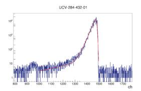
Fig. 4. Decay curve of the UCV scintillator for the 432 nm band under excitation at 284 nm.
