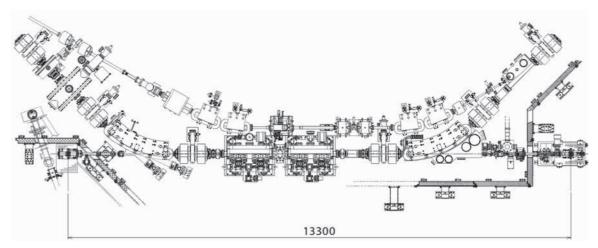
Fig. 1. Configuration of the free electron laser
