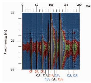
Fig. 1. Typical mass spectral intensities by photoionization of  $c-C_4F_8$  measured vacuum ultraviolet ranges from 10 to 30 eV.
