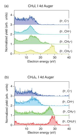
Fig. 1. PEPEPIPICO spectra of I 4d inner-shell photoionization at 100 eV for (a)  $CH_3I$  and (b)  $CH_2I_2$ .
