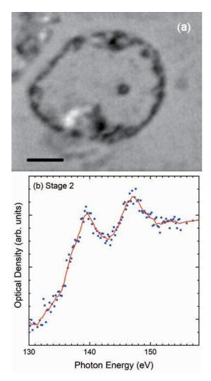
Fig. 1. X-ray absorption image, (a), and X-ray absorption spectrum, (b), of apoptosis nucleus in stage2 at P-L absorption edge. Bar is  $2 \mu m$  in length.
