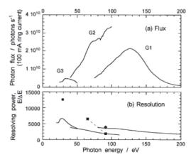
Fig. 1. Throughput from Dragon monochromator.
