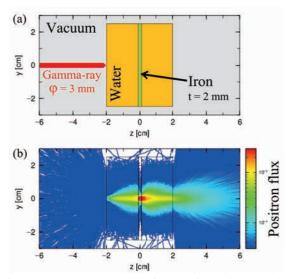
Fig. 2. (a) Geometry of the simulation model. (b) Calculated positron flux distribution.
