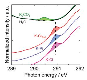
Fig. 1. Operando C-K edge XAFS spectra for Ni- $C_i$  electrocatalyst with exchanging the electrolyte solution between K- $C_i$  and K- $P_i$  by transmission mode at BL3U in the UVSOR synchrotron. The electrolyte aqueous solution of potassium carbonate was measured as reference compounds.
