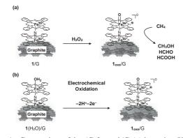
Fig. 1. Generation of  $\mathbf{1}_{oxo}$ /G from  $\mathbf{1}$ /G (a) by using  $H_2O_2$  or (b) by electrochemical oxidation.
