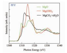
Fig. 2. Mg *K*-edge NEXAFS spectra of MgO, Mg(OH)<sub>2</sub> and MgCO<sub>3</sub>  $\cdot$  xH<sub>2</sub>O powder obtained from PFY mode.
