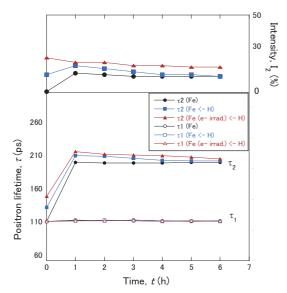
Fig. 2. Positron lifetimes and relative intensity  $I_2$  change after initial stress applied.
