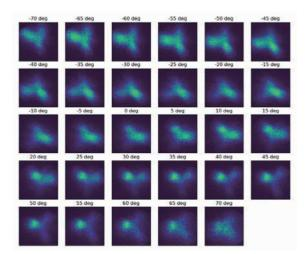
Fig. 2. ARPES intensity maps near the Fermi level as a function of the azimuth rotation. The photon of 7eV with a vertical polarization is used.
