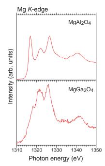
Fig. 1. Mg K-edge XANES spectra of  $MgAl_2O_4$  and  $MgGa_2O_4$
