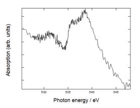
Fig. 2. O-K XAS spectrum for  $Ru_3(CO)_{12}$  (5 mg) in 5 ml CHCl<sub>3</sub> at room temperature.
