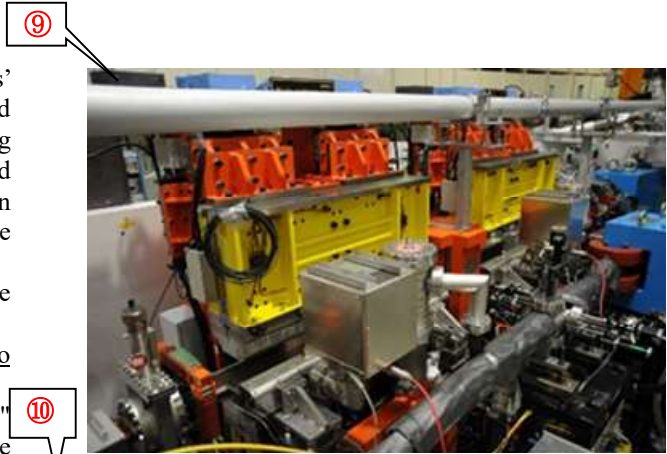
Fig. 1. Photo of the variably polarized U1 undulators in tandem.
