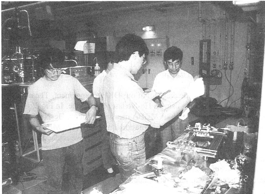
Prof. M. Kamada (right) and Dr. S. Kimura (middle) are installing gratings and mirrors on the exchange device of the SGM-TRAIN, with Dr. S. Hirose and Mr. M. Hasumoto (left).
