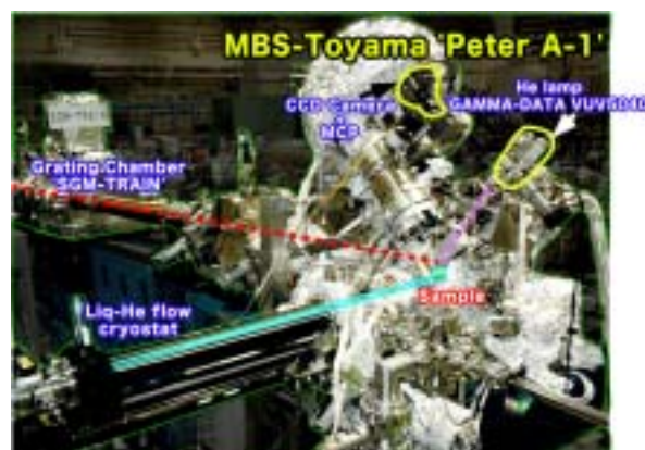
Fig. 2. High-resolution angle-resolved photoemission apparatus for BL5U
