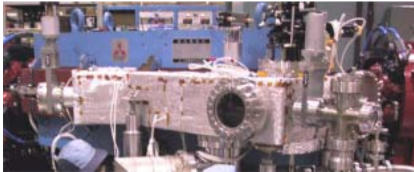
Fig. 2 New Bending Chamber for B6 just after the installation.
