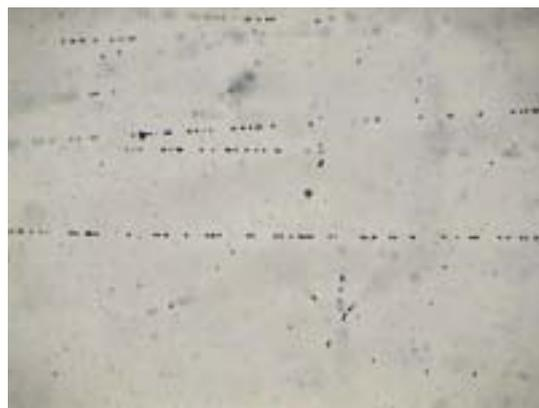
Fig. 1 A recorded trajectory of electron tracks. Horizontal scale is 120 microns.
