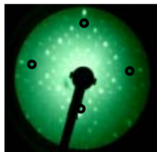
Fig. 1 LEED pattern of CuTTDPz film deposited on GeS(001) surface. Primary energy is 40 eV and the thickness of the film is 0.4 nm. The black circles in the figure represent diffraction spots from GeS(100).
