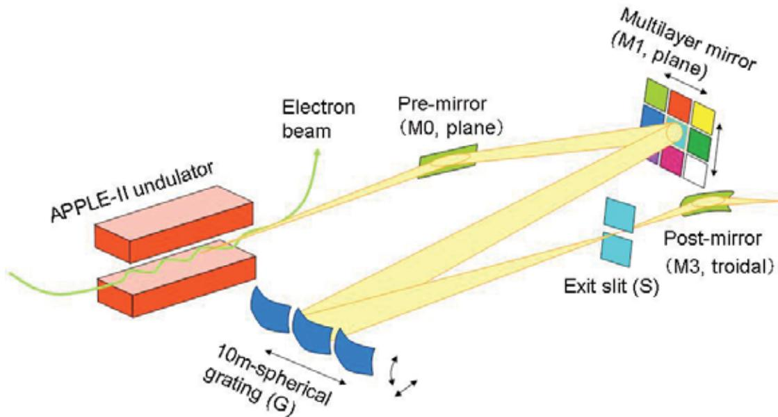
Fig.1. Schematic figure of BL7U.
