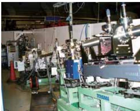
Fig .1 18-m spherical grating monochromator at BL2B.
