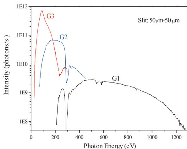
Fig. 1 Throughput from the VLS-PGM monochromator on BL4B.
