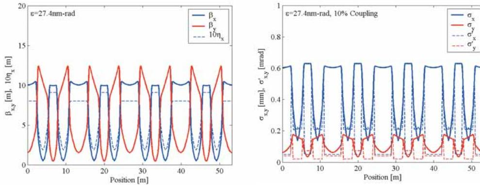
Horizontal/vertical betatron functions and dispersion function (left), and horizontal/vertical electron beam sizes and beam divergences (right) of UVSOR-II
