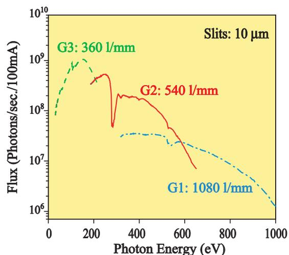
Fig. 2 Throughput of the monochromator at BL8B1.
