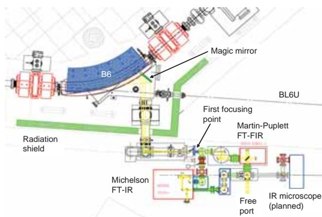
Fig. 2 Schematic figure of top view of BL6B.
