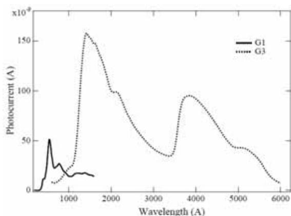
Fig. 1 Photocurrent at the sample position at BL1B.
