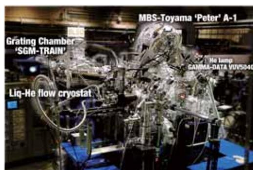
Fig. 2. High-resolution angle-resolved photoemission apparatus at BL5U
