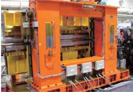
Fig. 1. Variable polarization U7 undulator.
