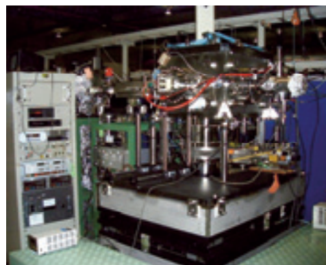
Fig. 2. End station of BL2B for gas phase spectroscopy of refractory materials.
