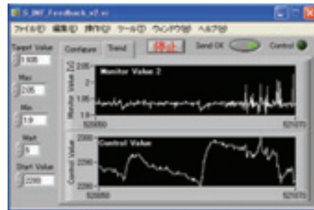
Fig. 3. The program for determining the set value of the electric septum used for the UVSOR-II injector.
