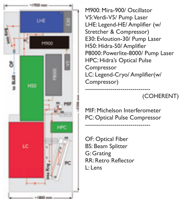
Fig. 1. A schematic drawing of the Ti:sapphire laser system.
