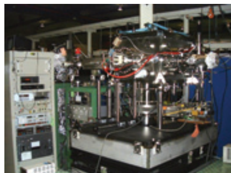
Fig. 2. End station of BL2B for gas phase spectroscopy of refractory materials.
