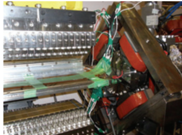
Fig. 2. Multi-wires installed in APPLE-II undulator.
