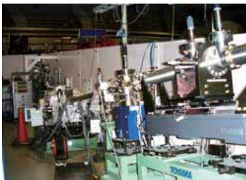
Fig. 1. 18 m spherical grating monochromator at BL2B.
