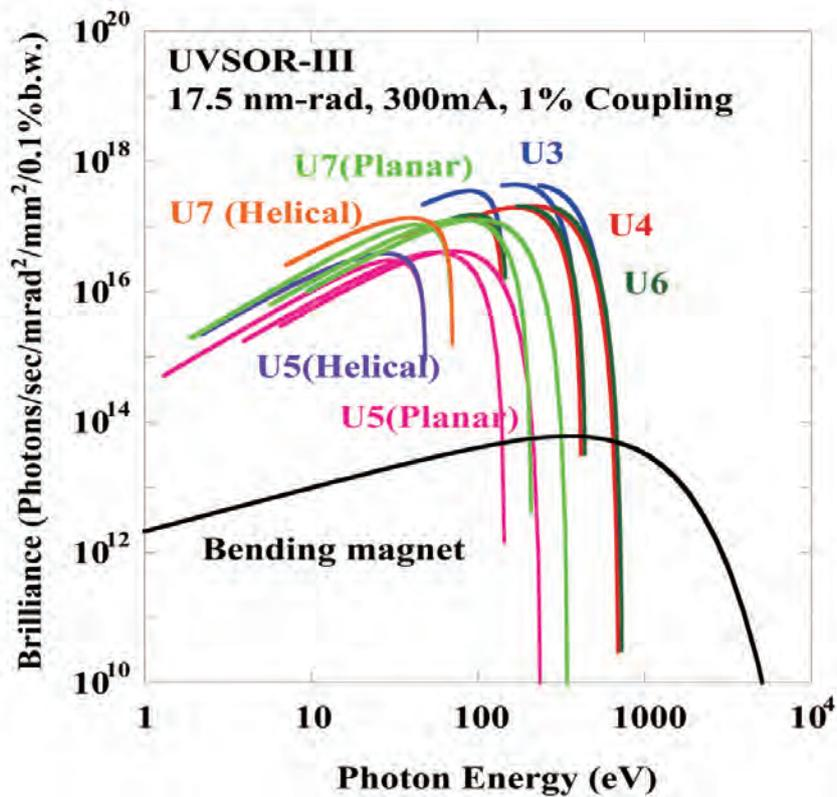
Brilliance of radiation from the insertion devices (U3, U4, U5, U6 and U7) and a bending magnet of UVSOR-III
