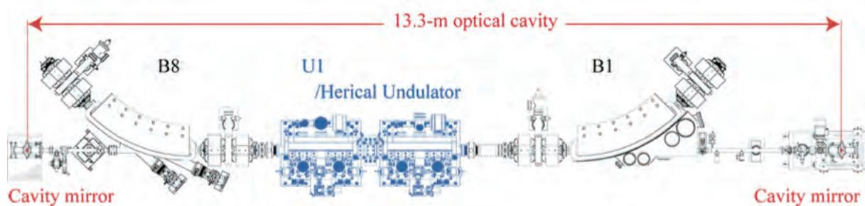
Fig. 1. Schematic of the 13.3 m-long optical cavity.
