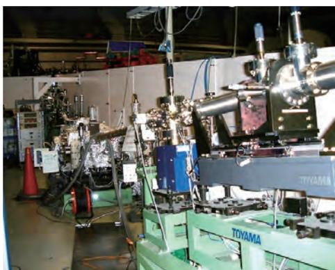
Fig. 1. 18 m spherical grating monochromator at BL2B.
