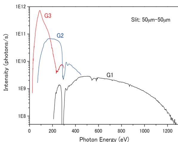
Fig. 1. Throughput from the VLS-PGM monochromator on BL4B.
