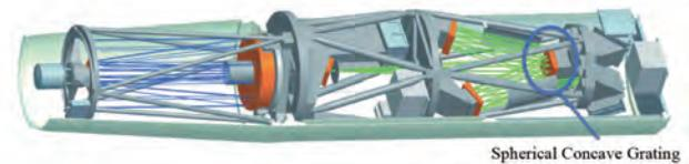
Fig. 1. Concave grating in the CLASP polarimeter.
