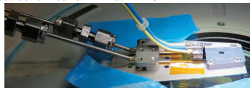
Fig. 1. photograph of the UVSOR in situ flow cell.
