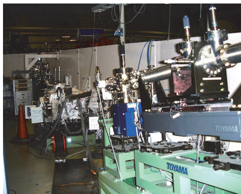
Fig. 1. 18 m spherical grating monochromator at BL2B.
