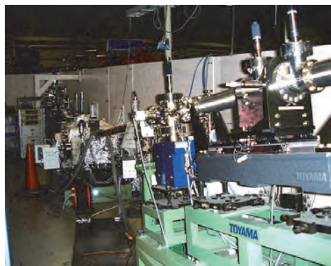
Fig. 1. 18 m spherical grating monochromator at BL2B.
