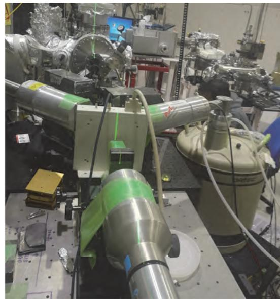
Fig. 1. BL1U LCS gamma-ray beamline with the setup for NRF-CT measurement.
