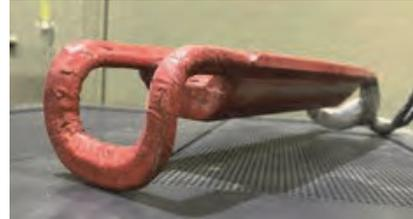
Fig. 2. Sextupole coil for multipole magnets.
