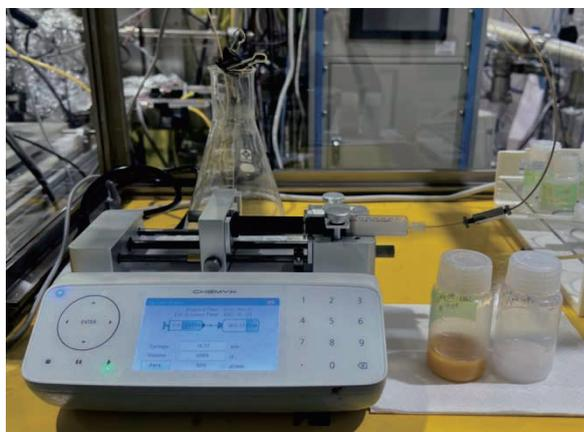
Fig. 1. Strontium-doped  $\text{NaTaO}_3$  photocatalyst particles suspended in water. White suspension in the syringe was sent to the liquid film cell for transmission XAFS measurements.
