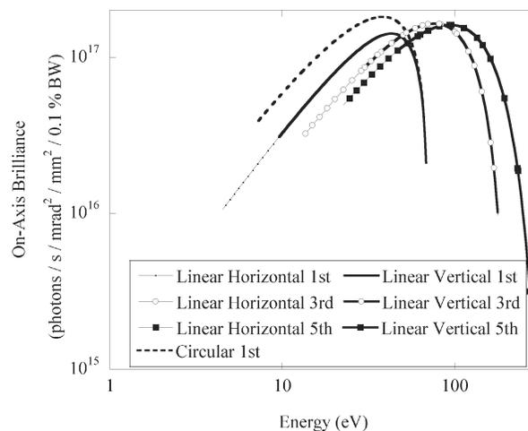
**FIGURE 2.** Brilliance spectra of the APPLE-II-type undulator of BL7U at UVSOR-II with the circular and linear polarizations at the beam current of 500 mA. 1-% coupling machine operation is expected in the calculation.
